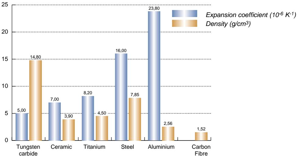
Thermal length increase in  $\mu$  with a 200mm probe extension and a temperature difference of 1K
