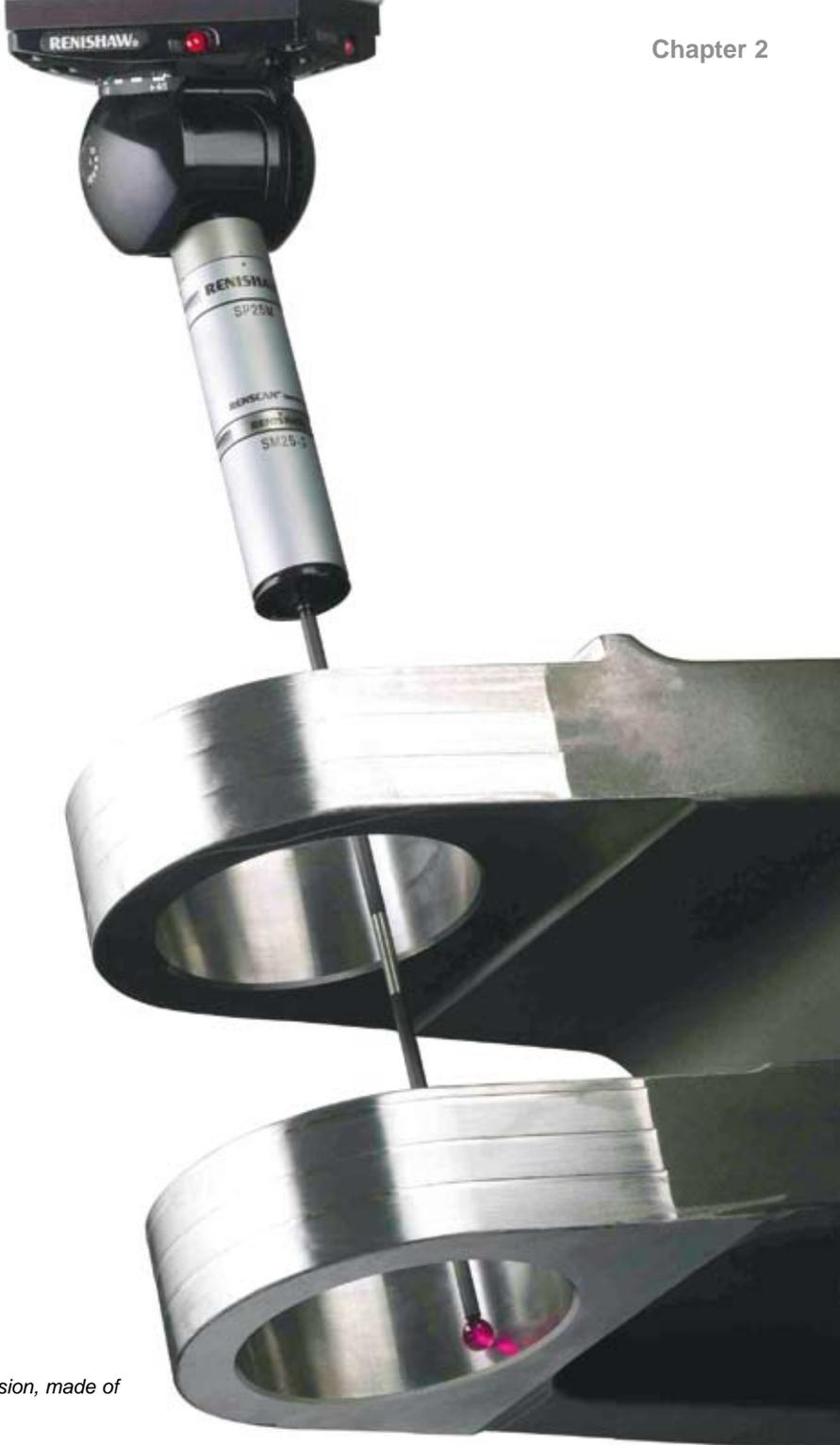
*Very long extension, made of carbon fibre*
