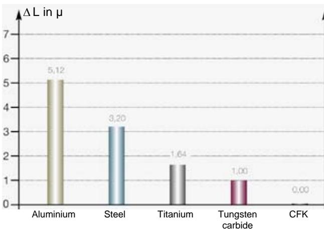
*Thermal length increase in μ with a 200 mm probe extension and a temperature difference of 1K*
