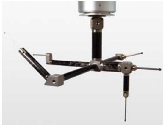
*A complex stylus configuration with multiple components*
