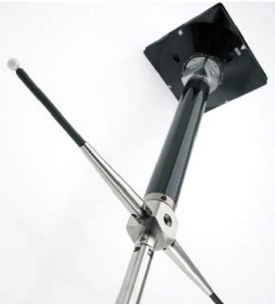
You can store the assembled adaptor plates in styli cabinets, or racks on the CMM and use them when needed. Whenever you make a change, there is no need to recalibrate the probe so you can start measuring immediately. With a probe rack, even highly complex work pieces can be measured in CNC mode.
