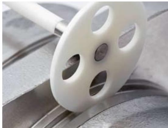
*Disc stylus for measuring edges or undercuts*
