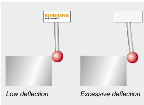
*Deflection has a direct impact on the accuracy of measurement*
